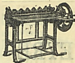
Millboard Cutter with Circular Knives
