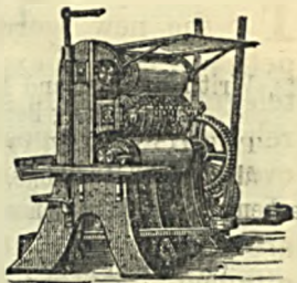
Calendar for Glazing Paper without Zinc-plates
